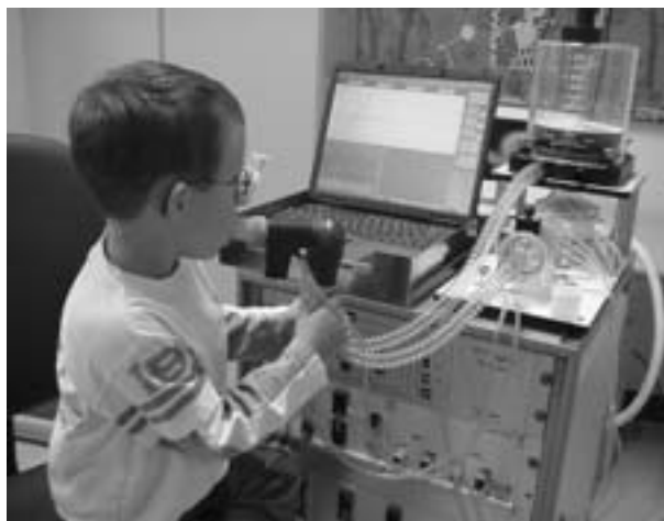
Fig. 8. – Rebreathing method in a closed system for measurements of diffusion capacity during quiet breathing.
